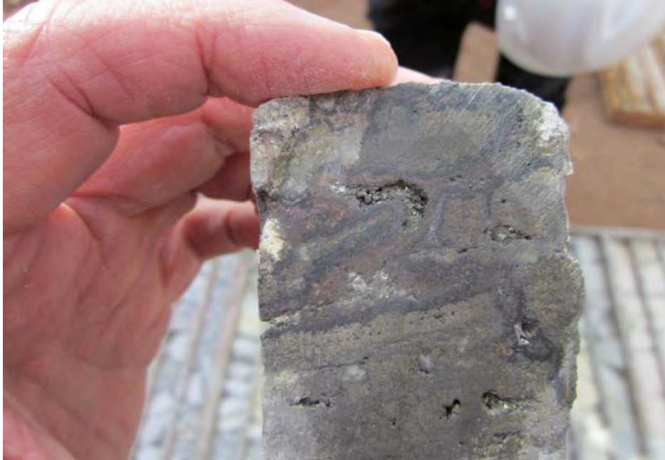
Figure 6.7: Crustiform Texture in HQ Core (~63.5 mm Width) - Pulacayo
