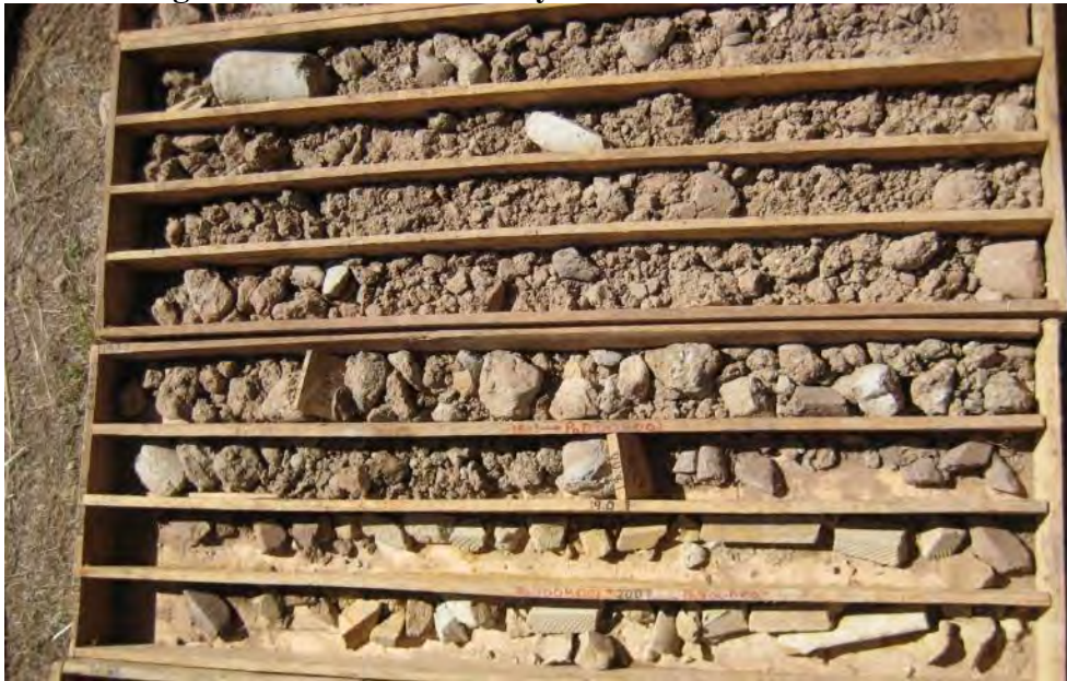
Figure 9.4: Poor Conglomerate Core Recovery in Paca Drill Hole PND-008
